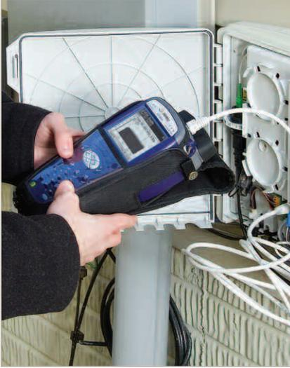
As deployment of FTTx and higher-speed digital subscriber line (DSL) and Internet Protocol (IP)-based triple-play services accelerates, the HST-3000 smoothly supports evolving service test requirements—from asymmetric DSL (ADSL) to ADSL2+ and very high bit-rate DSL (VDSL2) testing as well as the capability to add IPTV and VoIP testing. The HST-3000 can be upgraded in the field to support wideband copper qualification and trouble-shooting into the VDSL2 frequency range.
