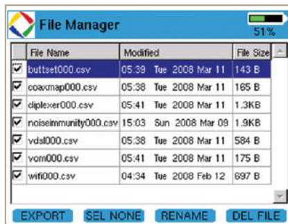
File Manager is used to rename, delete, or export result files from the SmartClass unit
